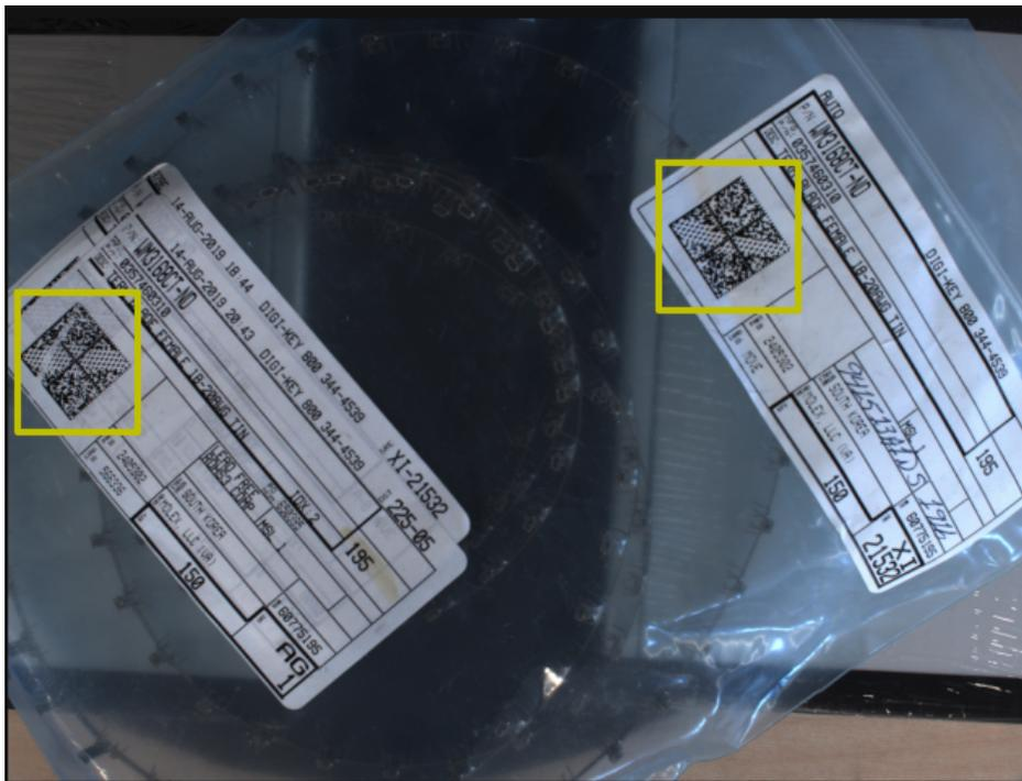
Figure 8: Validation image with bounding boxes shown. This example was contrived from random found items, intended to see if the model can generalize to entirely new examples. The two visible labels are almost entirely missed, with the model only able to find the QR codes on the label.
