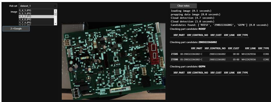
Figure 20: Another example of the custom tool. This board has considerably more text present on the board, but much of it can be excluded quickly as it is short and intended to label components on the board (for instance: ‘R25’ for ‘Resistor 25’). In this example, the system is again successful at finding the appropriate identification number and finds the entry in the database.
